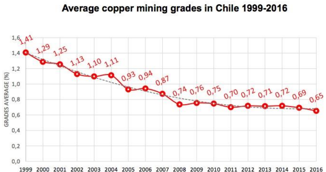
Fig. 7. Declining quality of Chilean copper resources. Source: Copper: Most Important Metal Were Running Short Of (streetwisereports.com)
